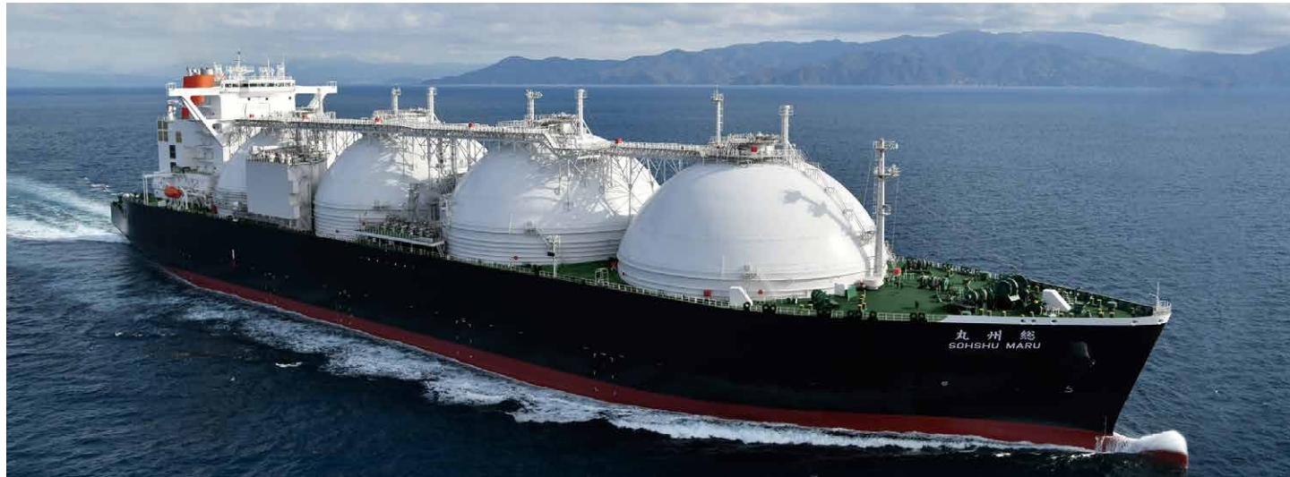
Transport ship SOHSHU MARU for marine transportation of LNG
