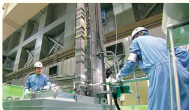
Acceptance inspection of MOX fuel
